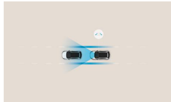
Lane Follow Assist (LFA): LFA helps prevent accidental lane departure and keeps your vehicle safely centered within the lane. Using a forward camera to recognise the intended lane, LFA will automatically provide corrective steering input to help maintain the centre path. This not only detects road lines but also the road edge.
