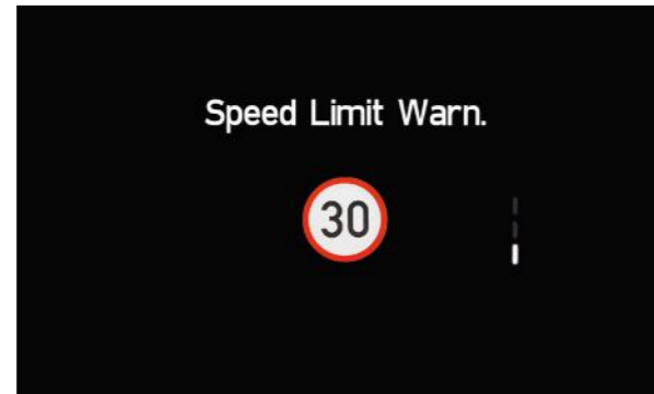
Intelligent Speed Limit Assist (ISLA): Information from the front cameras and navigation system identifies road speed limits and displays them in real time in the digital cluster.
