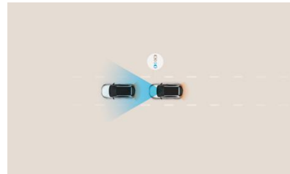
Forward Collision Avoidance (FCA): On detecting the risk of a collision with a forward vehicle, pedestrian or cyclist, the driver is alerted to the danger, and if necessary, brakes are automatically applied to help prevent a frontal collision.
