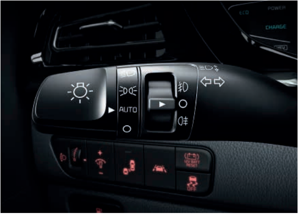
Automatic light control. Set the stalk to Auto and the headlights and tail lights come on automatically at dusk or in dark places.
