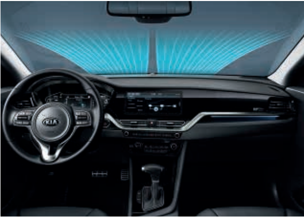
Auto defogger system. Sensors detect any condensation forming inside the front windscreen and automatically turn on the defogger for maximum visibility and safety.
